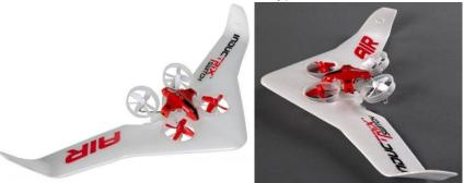
It is the Blade Inductrix Switch Air. It can actually be stripped of its wing, and the rear fans made horizontal if you want to use it as an normal quad, or with an additional part be reconfigured again as a hovercraft. They were delayed hitting the shops after first show in RCM&E, but are available now. Could be fun....
